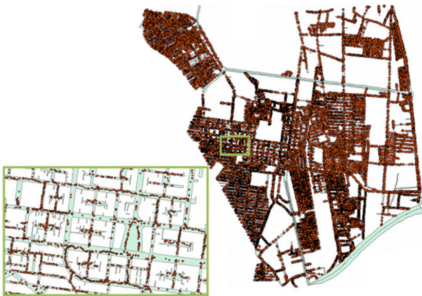
Fig. 2 Studied pavement network with locations of distress
